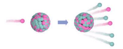
Neutrons produced by spallation – high energy beam on heavy metal target
