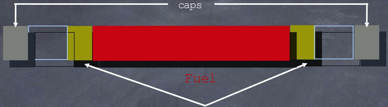
Y stabilized Zirconia ( $\text{ZrO}_2 + \text{Y}_2\text{O}_3$  (3 mole pc))
